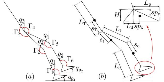
Fig. 1. Modelisation of the planar biped. a) Parameterisation of the biped. Note that angles are positive in counterclockwise. b) Length segments and position of the centers of mass.
