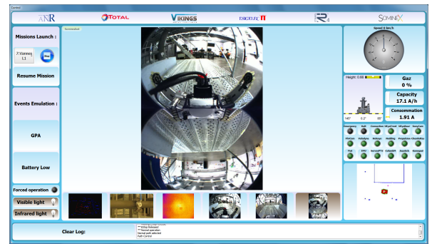
Fig. 4: Overview of the HMI. The HMI is dynamic according to the events encountered and the requests of the user. The operator can ask it to display on the central area: direct camera views, localization map, 3D map, path-planning, thermal image, etc.
