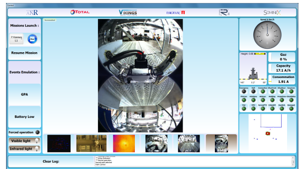
Fig. 4: Overview of the HMI. The HMI is dynamic according to the events encountered and the requests of the user. The operator can ask it to display on the central area: direct camera views, localization map, 3D map, path-planning, thermal image, etc.
