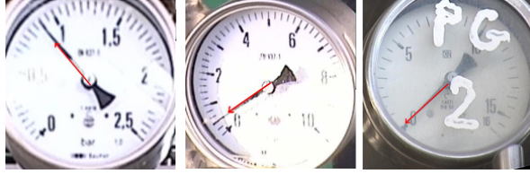
Fig. 8: Examples of correct needle detection in manometers in non-optimal conditions.
