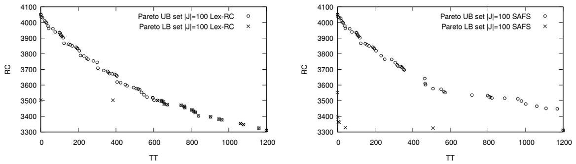
Figure 4: LB and UB sets returned by the B&B with the *Lex-RC* strategy (on the left panel) and with the *SAFS* strategy (on the right panel) for the  $RDD = 0.2$ ,  $TF = 0.6$  and  $id = 4$  instance with 100 jobs. The total tardiness is reported on the  $x$  axis, the rejection cost on the  $y$  axis. The UB set of the B&B is represented by round points and the LB set by x-shaped points.
