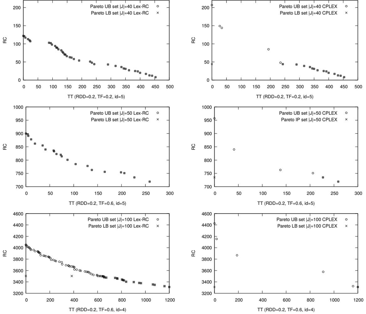
Figure 3: Pareto fronts from the B&B algorithm (on the left panels) and the  $\varepsilon$ -constrained approach (on the right panels) for three instances, respectively with 40 jobs (on top), 50 jobs (second row) and 100 jobs (last row). The total tardiness is reported on the  $x$  axis, the rejection cost on the  $y$  axis. The UB set of the B&B is represented by round points and the LB set by x-shaped points. The features of each instance are referenced below each figure.
