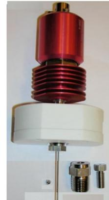
(c) Capillary sampler
