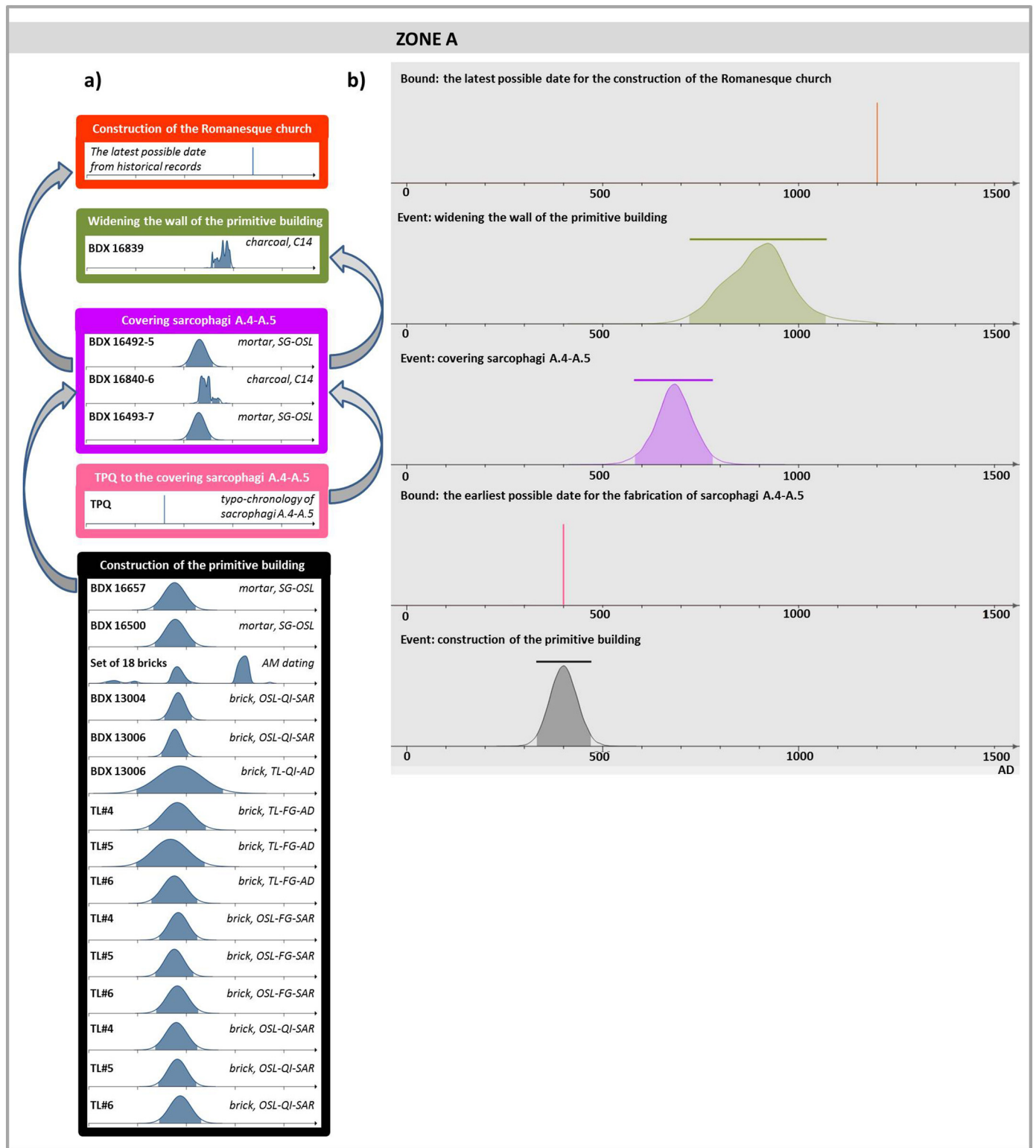
Fig. 7. Procedure and results of the statistical combination (95% confidence level) of all the dating results obtained for the samples originating from zone A.
