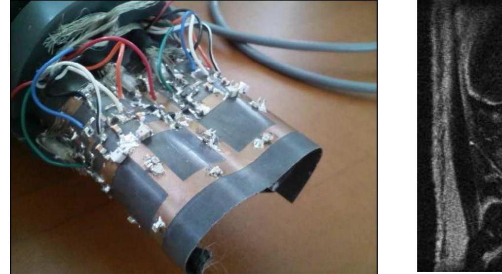
Fig. 1: Four-channels array coil designed for simultaneously image both knees\*
