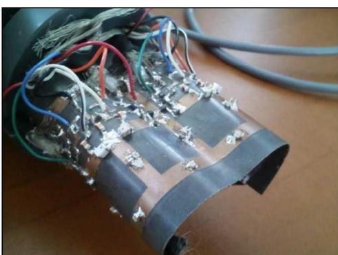
Fig. 1: Four-channels array coil designed for simultaneously image both knees\*
