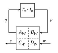
Fig. 1. Block Diagram of an identical dissipative systems interconnection
