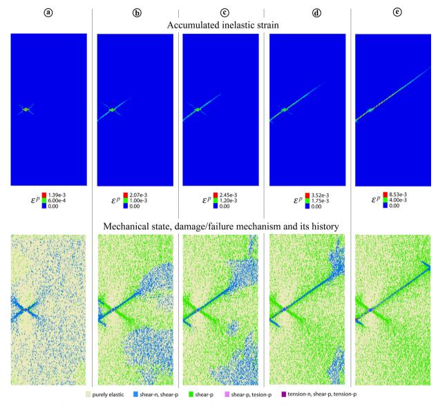
Fig. 11. Evolution of the  $\varepsilon^p$  and mechanical state patterns in the model with Gaussian distribution of  $\nu$  and a weak zone with  $\sigma_t$  = 0.03 MPa;  $k_c$  = 0.3 MPa. The initial stresses correspond to point 4 in Fig. 3a ( $\sigma_2$  =  $\sigma_1$  = 0.66 MPa).
