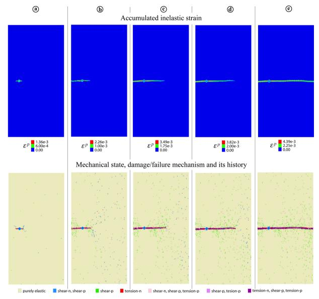
**Fig. 9.** Evolution of the  $\varepsilon^p$  and mechanical state patterns in the model with a Gaussian distribution of  $\nu$  and a weak zone with following strength parameters:  $\sigma_t = 0.03$  MPa;  $k_c = 0.3$  MPa. The initial stresses and boundary conditions are the same as in the two previous models (the stress state corresponds to point 2 in Fig. 3a).
