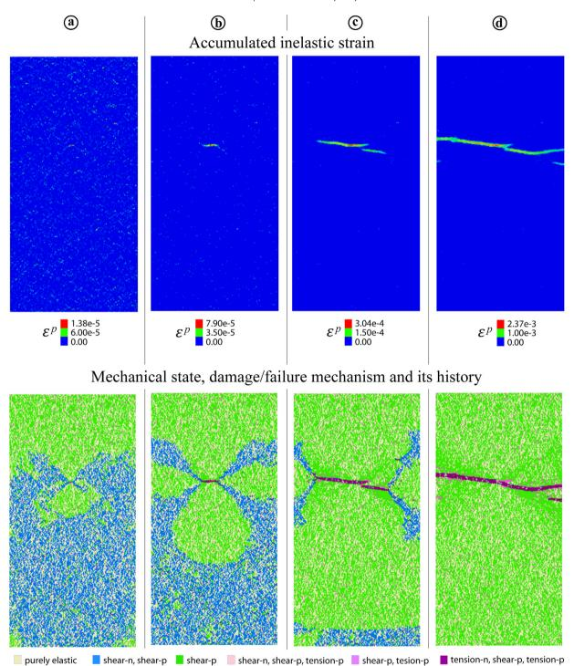
Fig. 8. Evolution of the  $\varepsilon^p$  and mechanical state patterns in the model with a Gaussian distribution of  $\nu$ . The initial stresses and boundary conditions are the same as in the previous model (the stress state corresponds to point 2 in Fig. 3a).
