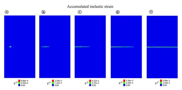
Fig. 5. Evolution of the  $\varepsilon^p$  pattern in the model with Gaussian  $\nu$  distribution and a weak zone with the reduced initial strength parameters:  $\sigma_t = 0.03 \text{ MPa}$ ;  $k_c = 0.1 \text{ MPa}$ . The initial stresses and boundary conditions are the same as in the previous model.
