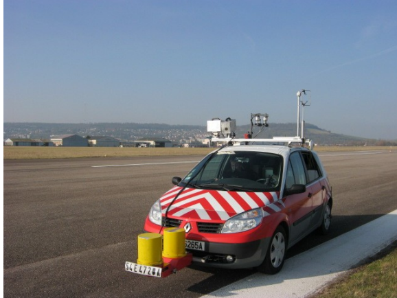
Figure 1: Instrumented vehicle used for mobile measurements within Local Climate Zones
