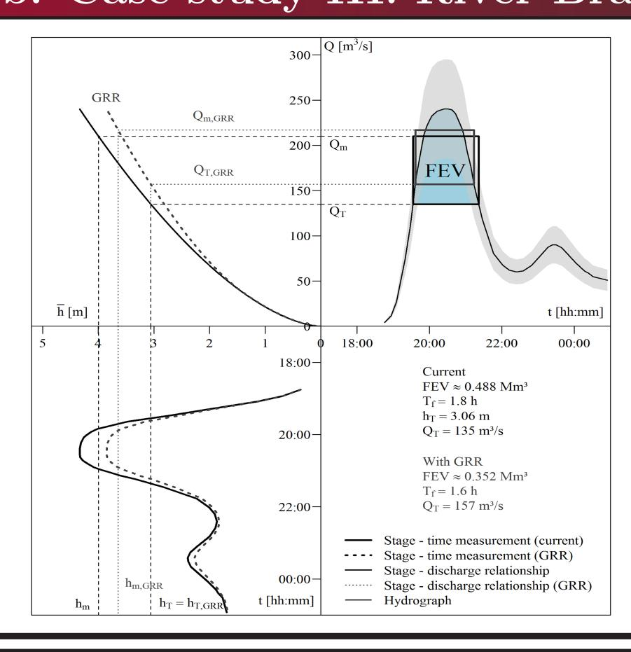
An alternative to raising flood walls: giving room to the river (GRR) increases the river width in order to increase the discharge capacity for a similar water depth.
