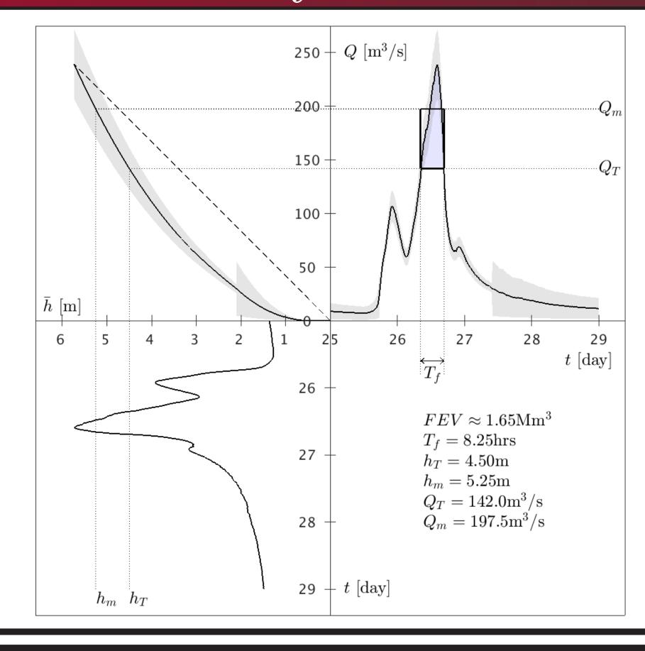
Exploratory flood-alleviation scheme comprising (i) temporary storage in reservoirs, (ii) upscaled 'leaky' debris dams, and (iii) tree planting:
