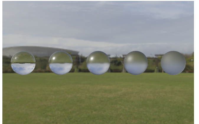
Figure 4. Surface scattering axis. The roughness increases from the left-most object to the right-most one. The absorbance is zero along this axis.
