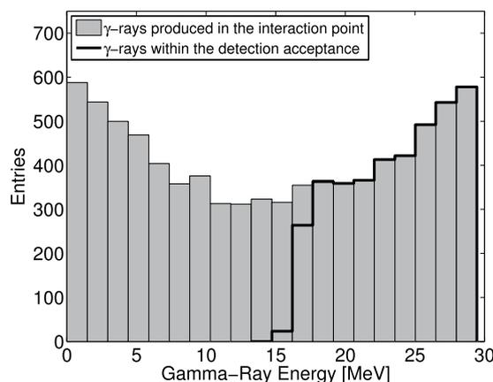
**Figure 7.** Computed energy spectrum of the  $\gamma$ -rays produced by Compton scattering of a 1034 nm laser beam off a 1.28 GeV electron beam. Only the  $\gamma$ -rays with energies above 15 MeV are detected resulting in the average energy of the measured  $\gamma$ -rays being 24 MeV.
