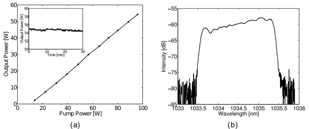
**Figure 5.** (a) Output power versus the pump power of the amplified laser beam. (b) Emission spectrum of the amplified laser beam. The square shape of the emission spectrum is due to the transmission bandwidth of the stretcher and compressor couple.
