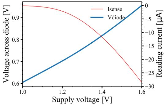
Figure 4: Dependence of voltage supply on reading current
