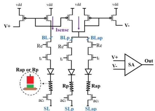
Figure 3. Circuit state in array read mode
