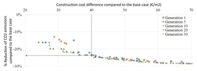
Fig. 8 Pareto frontier for CO<sub>2</sub> emissions and construction cost (case study)
