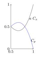
The power P should be superior to the thrust power  ${\cal F}_x$  in order that additional energy to be produced.
