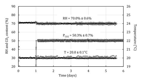
Figure 4: Temperature, RH and  $CO_2$  content during a preliminary test conducted at  $20^{\circ}$ C, 70% RH and 50%  $CO_2$ . The first reported number represents the average for each measurement, whereas the second represents the standard deviation.
