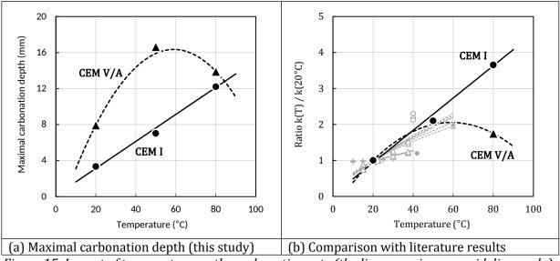
Figure 15: Impact of temperature on the carbonation rate (the lines are given as guidelines only)
