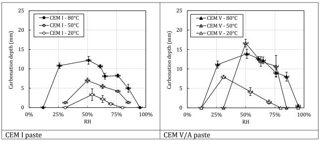
Figure 12: Carbonation depth versus RH
