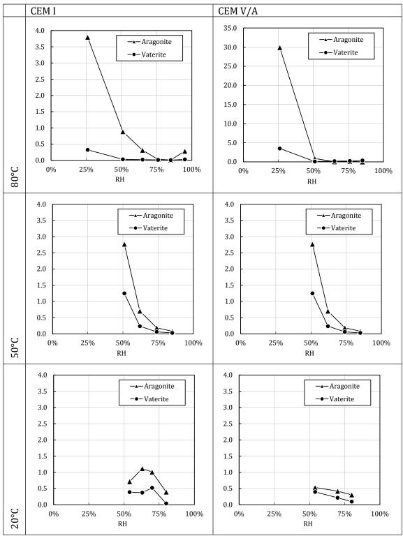
Figure 11: Polymorphic abundance of calcium carbonate assessed using XRD and the RIR method: ratio  $(\bar{x}_i/\bar{x}_c)$  as a function of temperature and RH
