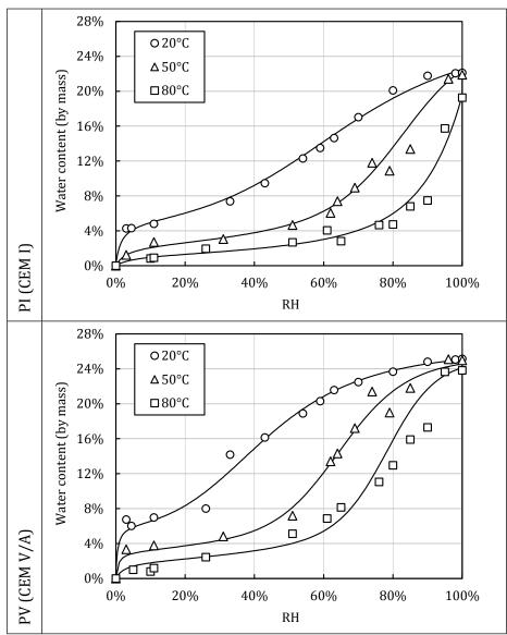
Figure 6: Desorption isotherm of the hardened pastes as a function of temperature (the solid lines are provided as guidelines only) [31]
