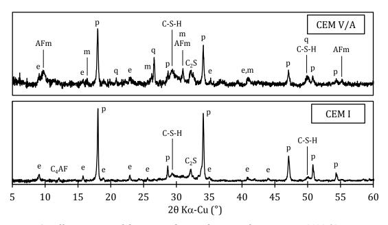
Figure 5: Diffractograms of the non-carbonated pastes after curing at  $20^{\circ}$ C (AFm = monosulfoaluminate;  $C_2$ S = dicalcium silicate;  $C_4$ AF = calcium aluminoferrite;  $C_7$ C-S-H = calcium silicate hydrates;  $C_7$ C-S-H = calcium silicate hydrates h
