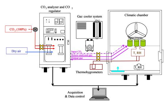
Figure 3: Device for accelerated carbonation tests
