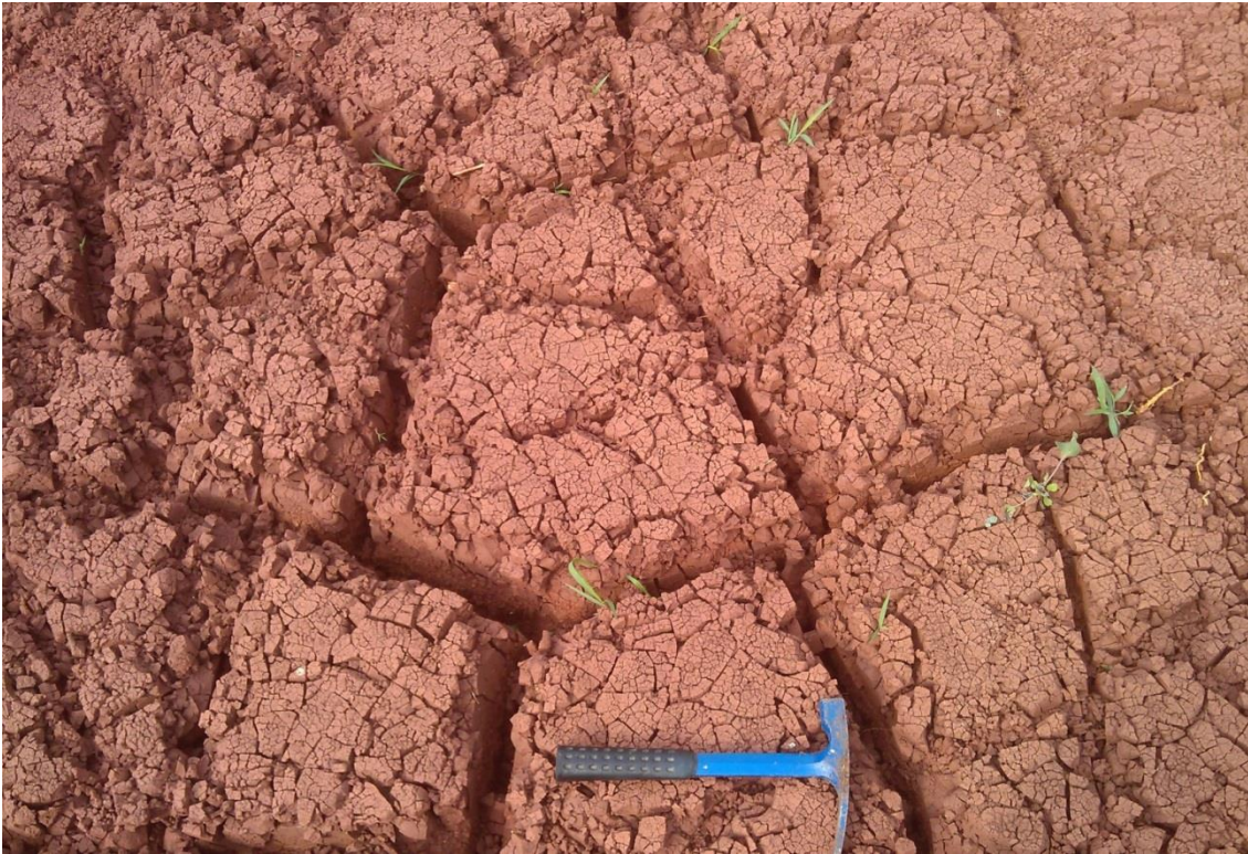
Figure 1. Desiccation crack polygon in natural soil.
