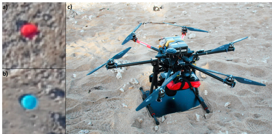
Figure 4. (a) Example of red target used as Ground Control Point. (b) Example of blue target used as check point to assess the quality of the reconstructed DEM. (c) DRELIO 10, Unmanned Aerial Vehicle (UAV) designed from a hexacopter platform 80 cm in diameter.
