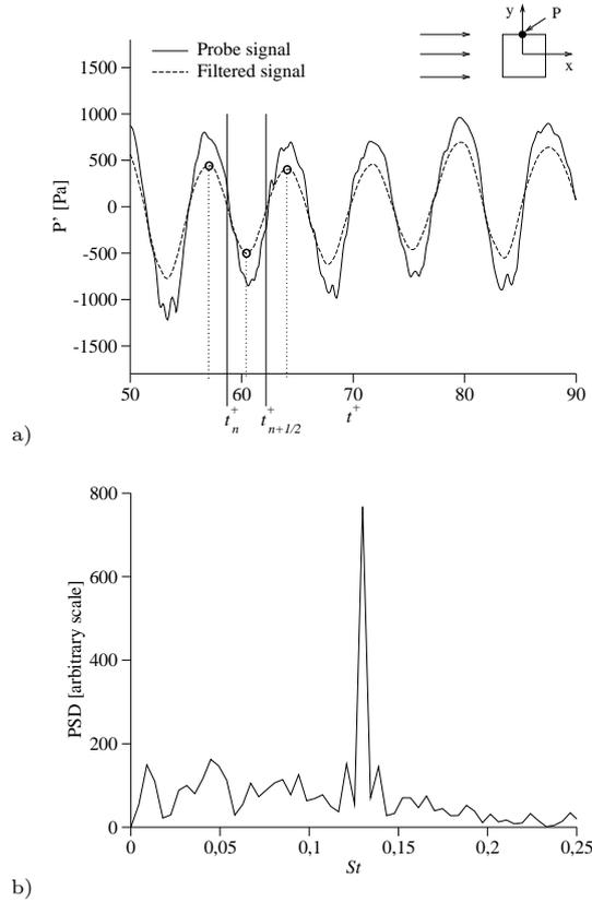
**Fig. 6 Definition of the vortex shedding phase for case *LES-WF*: (a) sample of the unfiltered pressure fluctuation (after removing the mean value) and low-pass filtered pressure as a function of the non dimensional time  $t^+ = t_{LES}/t_c$ . (b) FFT of the unfiltered pressure signal.**
