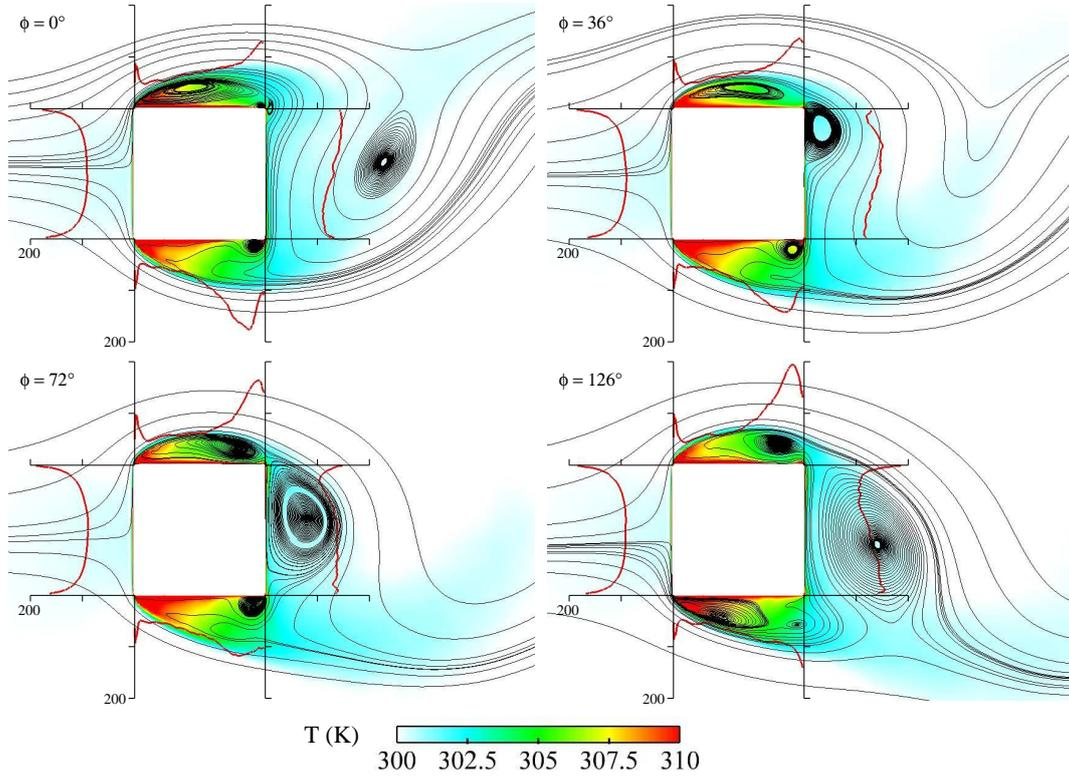
**Fig. 20** Phase-averaged quantities taken at four selected phase angles of case *LES-WR*: Nusselt number profiles at each side of the cylinder (scales are all identical), velocity stream lines and flow temperature distribution.
