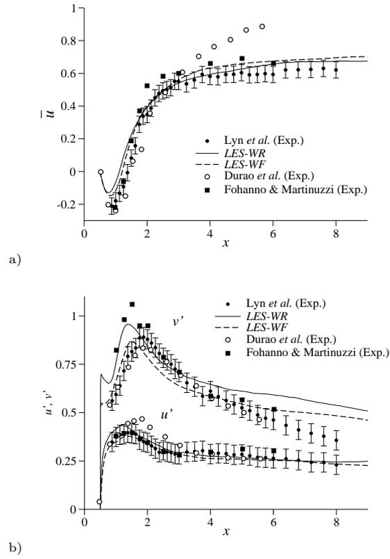
Fig. 11 Longitudinal profiles of time-averaged streamwise velocity,  $\bar{u}$ , in the wake of the cylinder (cut  $Y_0$  of Fig. 7) (a). Corresponding streamwise,  $u'$ , and transverse,  $v'$ , velocity fluctuations (b). Experimental results of Lyn *et al.* [11] ( $\bullet$ ), Durao *et al.* [13] ( $\circ$ ) and Fohanno and Martinuzzi [23] ( $\blacksquare$ ) and present numerical results for cases *LES-WR* (—) and *LES-WF* (---).
