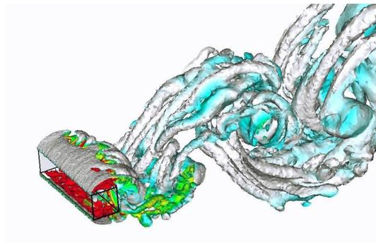
**Fig. 9** Iso-surface of vorticity colored by temperature (case *LES-WF*).
