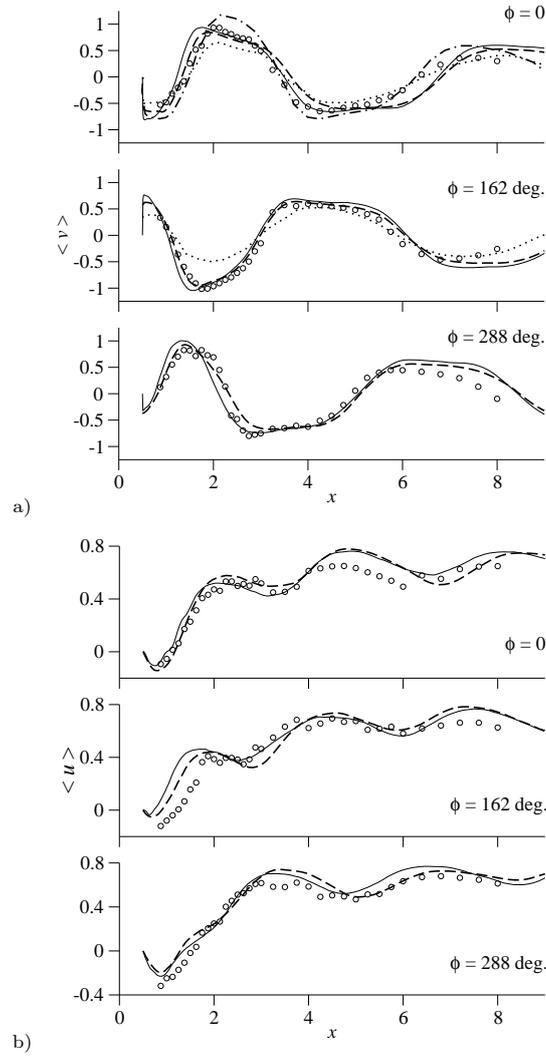
**Fig. 14** Longitudinal profiles of phase-averaged transverse velocity,  $\langle v \rangle$ , (a) and streamwise velocity,  $\langle u \rangle$ , (b) in the wake of the cylinder at three selected phase angles: experimental results of Lyn *et al.* [11] ( $\circ$ ), LES results of Liou *et al.* [7] ( $\cdots$ ), case KAWAMU in Rodi *et al.* [4] ( $-\cdot-\cdot-$ ) and present results for cases *LES-WR* ( $-\cdot-$ ) and *LES-WF* ( $----$ ).
