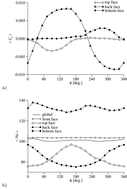
**Fig. 21** Space-averaged value of the phase-averaged algebraic friction coefficient,  $\langle C_f \rangle$ , (a) and Nusselt number,  $\langle Nu \rangle$ , (b) on different faces of the cylinder as a function of the phase  $\phi$ .
