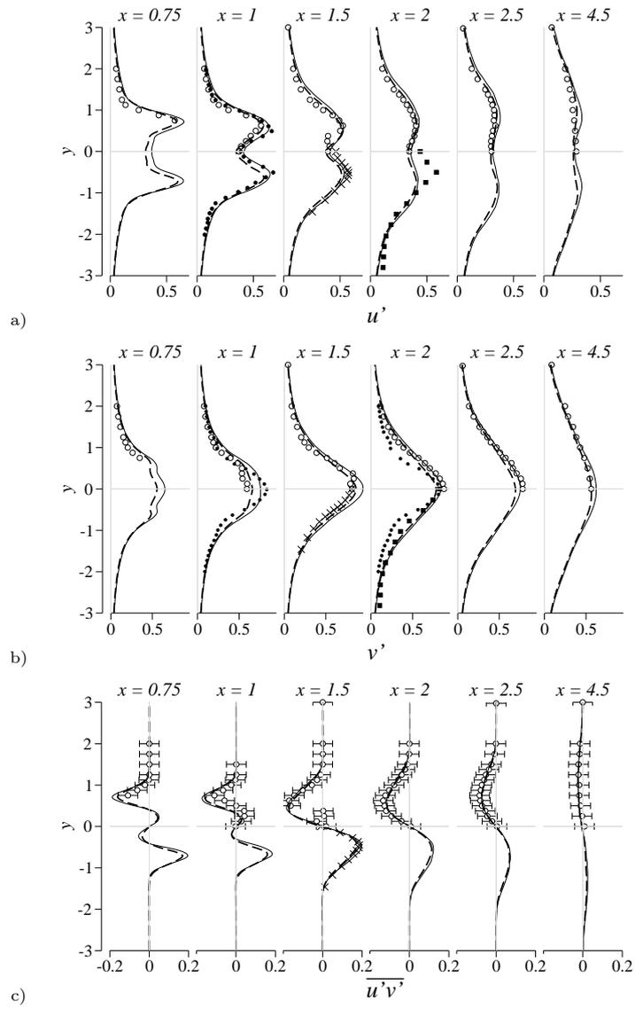
**Fig. 13** Transverse profiles of time-averaged streamwise velocity fluctuation,  $u'$ , (a), transverse velocity fluctuation,  $v'$ , (b) and velocity correlation,  $\overline{u'v'}$ , (c) in the wake of the cylinder. Symbol legend: same as Fig. 12 and experimental results of Durao *et al.* [13] (■).
