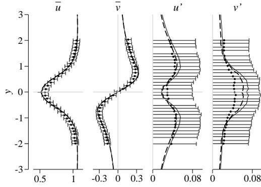
**Fig. 8** Transverse profiles of time-averaged streamwise velocity,  $\bar{u}$ , transverse velocity,  $\bar{v}$ , streamwise velocity fluctuation,  $u'$ , and transverse velocity fluctuation,  $v'$ , upstream the cylinder at  $x = -1$  (cut  $X-1$  of Fig. 7): experimental results of Fohanno and Martinuzzi [23] ( $\bullet$ ) and present numerical results for cases *LES-WR* (—) and *LES-WF* (---).
