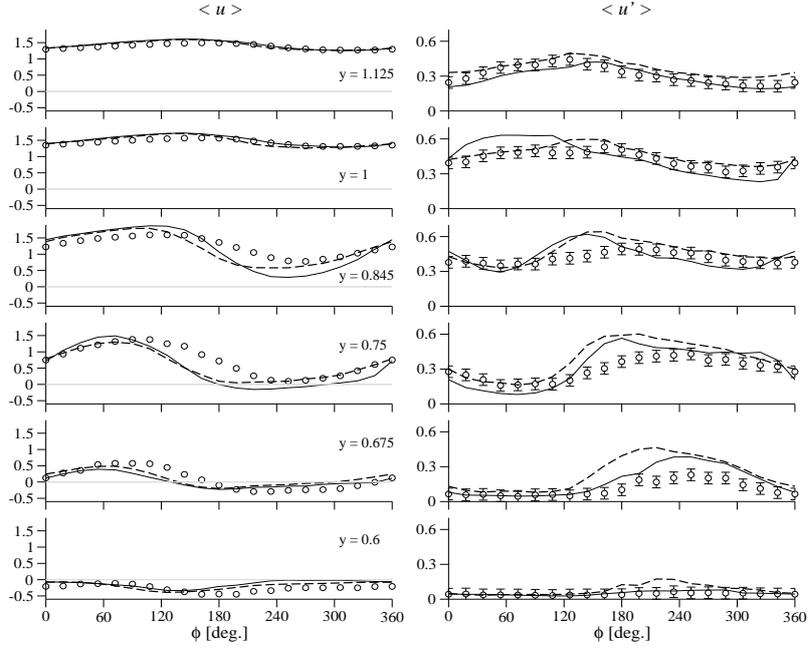
**Fig. 18** Evolution of phase-averaged streamwise velocity,  $\langle u \rangle$ , and fluctuation,  $\langle u' \rangle$ , as a function of the phase at six selected vertical positions above the top side of the cylinder ( $x = 0.25$ ): experimental results of Lyn and Rodi [10] (o) and LES results for cases *LES-WR* (—) and *LES-WF* (---).
