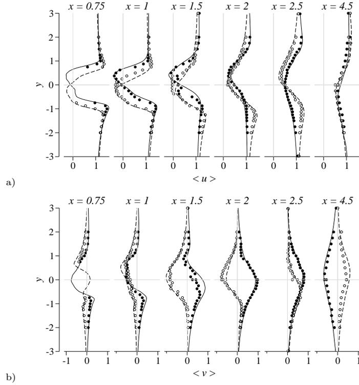
Fig. 16 Transverse profiles of phase-averaged streamwise velocity,  $\langle u \rangle$ , (a) and transverse velocity,  $\langle v \rangle$ , (b) in the wake of the cylinder at two selected phase angles: experimental results of Lyn *et al.* [11] at  $\phi = 0^\circ$  (o) and  $108^\circ$  (●) and present results for case *LES-WR* at  $\phi = 0^\circ$  (—) and  $108^\circ$  (----).
