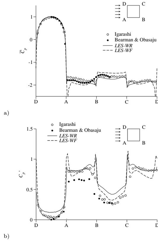
**Fig. 10** Profiles of time-averaged pressure coefficient,  $C_p$ , (a) and fluctuation,  $C_p'$ , (b) around the cylinder walls for the two LES cases compared to the experimental data of Igarashi [24] and Bearman and Obasaju [12].
