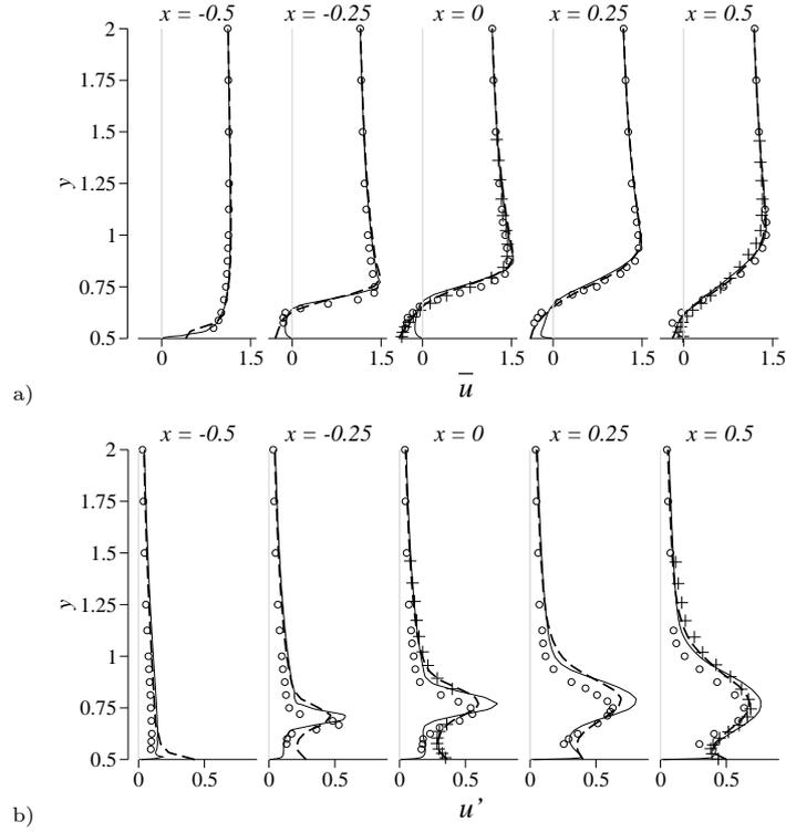
**Fig. 17** Transverse profiles of time-averaged streamwise velocity,  $\bar{u}$ , (a) and fluctuation,  $u'$ , (b) on the top face of the cylinder (cuts  $X=-0.5$  to  $X=0.5$  of Fig. 7): experimental results of Lyn and Rodi [10] ( $\circ$ ), LES results of Hangan and Kim [25] ( $+$ ) and present LES results for cases *LES-WR* (—) and *LES-WF* (----).
