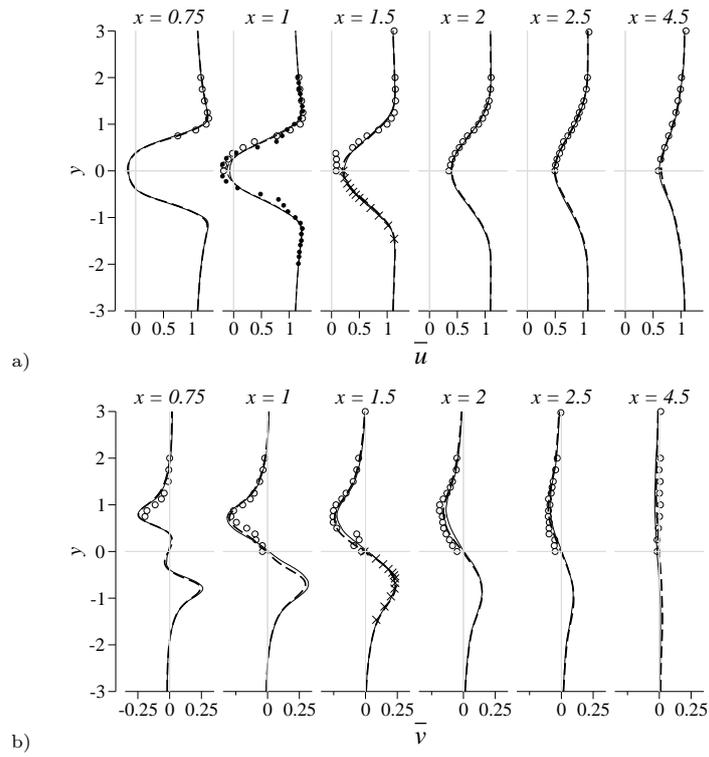
**Fig. 12** Transverse profiles of time-averaged streamwise velocity,  $\bar{u}$ , (a) and transverse velocity,  $\bar{v}$ , (b) in the wake of the cylinder (cut  $X_{0.75}$  to  $X_{4.5}$  of Fig. 7): experimental results of Lyn *et al.* [11] ( $\circ$ ), Fohanno and Martinuzzi [23] ( $\bullet$ ), LES results of Hangan and Kim [25] ( $\times$ ) and present numerical results for cases *LES-WR* (—) and *LES-WF* (- - -).
