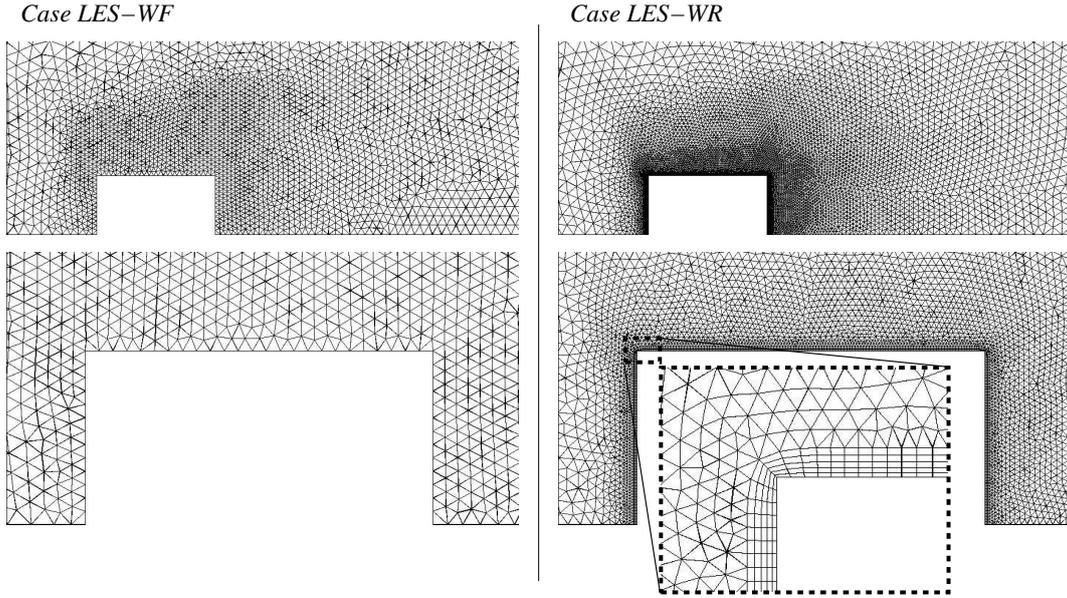
Fig. 3 Zooms on the side view of the top half of the two unstructured grids: full tetrahedral grid (case *LES-WF*) and hybrid prismatic/tetrahedral grid (case *LES-WR*). Bottom right image is a zoom on the five layers of prismatic elements.
