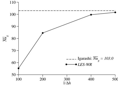
Fig. 4 Global Nussel number of the cylinder,  $\overline{Nu}_g$ , for the wall-resolved case (*LES-WR*) as a function of the mesh wall resolution  $1/\Delta h$  compared to the experimental correlation of Igarashi [14] (Eq. (14))
