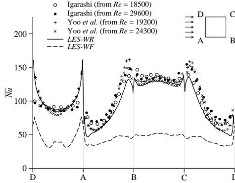
**Fig. 19** Profiles of time-averaged local Nusselt number,  $\overline{Nu}$ , around the cylinder walls : experimental results of Igarashi [14] ( $\circ$  and  $\bullet$ ) and of Yoo *et al.* [15] ( $+$  and  $\times$ ) scaled using Eq. (15) and compared to the present LES results (— and - - -).
