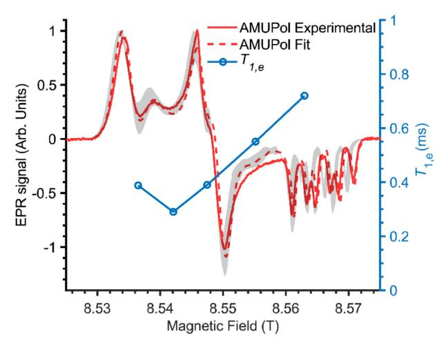
**Fig. 4.** High-field EPR spectrum of 10 mM of AMUPol in  $D_8$ -glycerol/ $D_2O/H_2O$  (60/30/10 v%) + 2M  $^{13}C$ -urea, recorded at 100 K, for a microwave frequency of 240 GHz. The red curve represents the experimental spectrum and the red dashed line represents the theoretical EPR spectrum obtained with fitted parameters reported table 1. The blue dots correspond to the measured electron spin-lattice relaxation times,  $T_{1e}$  (right axis).
