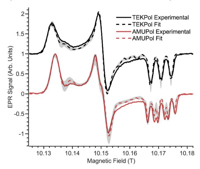
**Fig. 3.** High-field EPR spectra of 15 mM TEKPol in CHCl $_3$ /TBE/MeOH-D $_4$  (65/35/5 v%) (black) and 10 mM AMUPol in D $_8$ -glycerol/D $_2$ O/H $_2$ O (60/30/10 v%) + 2M  $^{13}$ C-urea (red), both recorded at 100 K with a microwave frequency of 285 GHz. Best fits obtained from the DFT-calculated parameters are shown with black and red dashed lines for TEKPol and AMUPol, respectively. The grey overlays represent the errors reported in Table 1.
