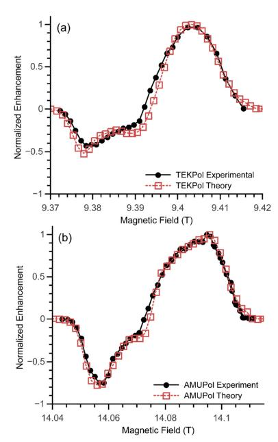
Fig. 5. Experimental (black circles) and simulated (red squares) MAS-DNP field profiles, i.e. the enhancement  $\epsilon_{\text{on/off}}$  as a function of the magnetic field while keeping the  $\mu$ w irradiation frequency constant, for TEKPol (a) and AMUPol (b) at 9.4 T and 14.1 T, respectively.
