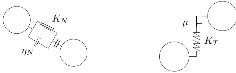
Figure 11. Rheological elements schematizing contact behavior: normal force (left) combines a spring (possibly nonlinear, with K_N depending on elongation), a viscous dashpot, and a no-tension joint (no adhesion here). The tangential law (right) involves a plastic slider.
