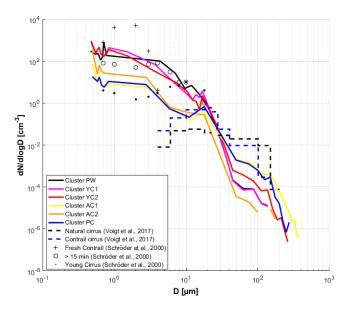
**Figure 7.** Number particle size distribution for each cluster including all data points of all flights. FSSP-300 measurements are from 0.5 to  $17 \,\mu\text{m}$  and 2DC measurements from 50 to  $800 \,\mu\text{m}$ . The data are linearly interpolated in logarithm space in the gap between 17 m and 50  $\mu\text{m}$ .
