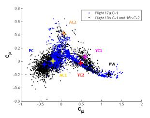
**Figure 5.** Example of data projection in the  $C_{j2}-C_{j3}$  space where data from flight 17a (blue data points) are superposed on the data from the benchmark flights 19b and 16b (black data points).
