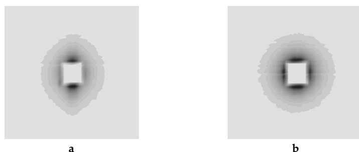
Figure 20. Small angle neutron scattering records (halo) of 1 pass AZ31 at RT for (a)—39 and (b)—8 m as distances sample to detector.
