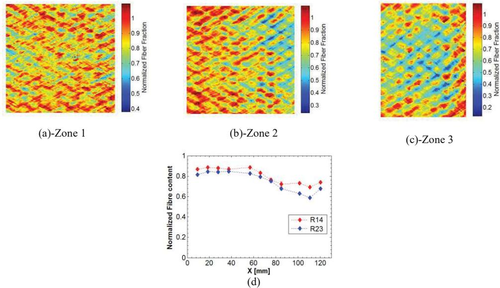
**FIGURE 5 :** 280°C-specimen. Fiber content  $\bar{\phi}$  maps of Zone 1 (a), 2 (b) and 3 (c). (d) Fiber content  $\bar{\phi}$  variation along the horizontal direction (referring to Fig. 2 in rows 1-4 and 2-3).
