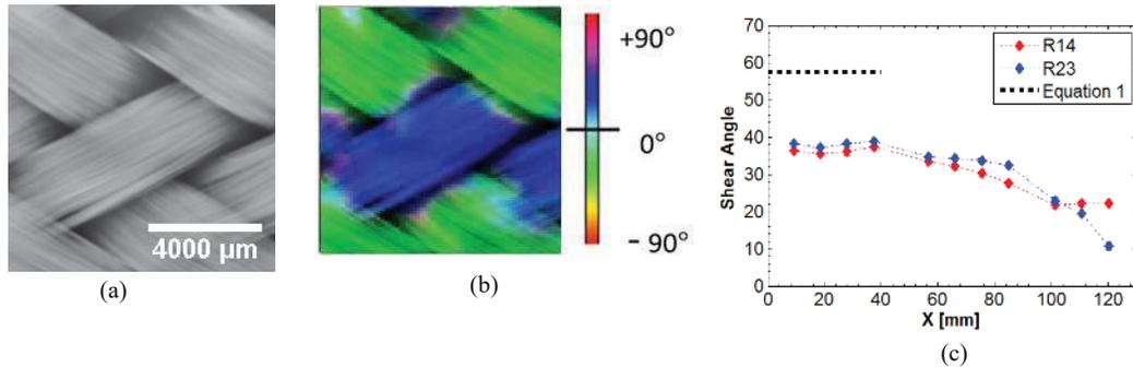
FIGURE 4: 280°C-specimen. (a) Typical REV. (b) Orientation map. (c) Evolution of the local shear angle as a function of the horizontal position of the REV along the tested specimen.
