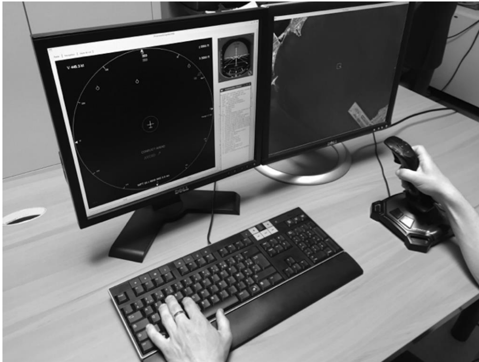
Figure 1. Schematic representation of the apparatus during the experiment. The Supervision task is displayed on the left screen and the Tracking task on the right screen.
