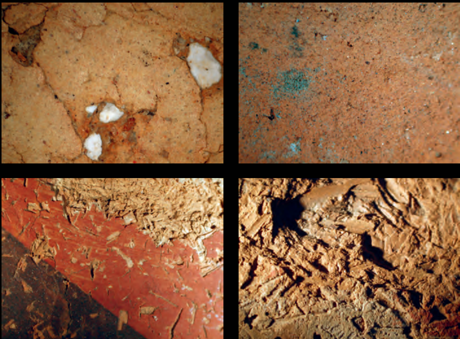
2 Examples of different kinds of filler observed under stereomicroscope. a-b: mineral filler; c-d: organic filler [straw] (photo: A. Dupont-Delaleuf, MAFTur).
