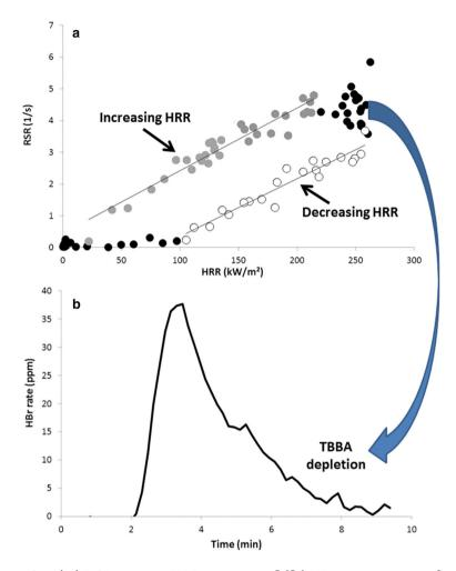
Figure 10. (a) RSR versus HRR curve and (b) HBr rate versus time for PE filled with 10 wt% of TBBPA.
