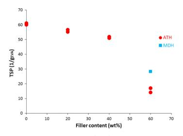
Figure 7. Total smoke release in  $m^2/m^2$  per gram of EVA versus filler content for various EVA filled with ATH and MDH.
