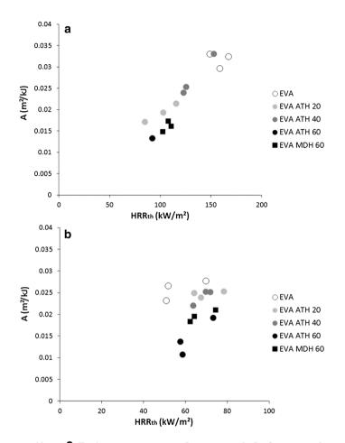
Figure 9. A (in  $m^2/kJ$ ) versus  $HRR_{th}$  for materials from series C (a HRR increasing; b HRR decreasing).
