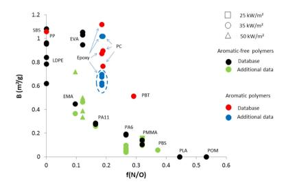
Figure 5. B  $(m^2/g)$  versus f(N/O) weight fraction for the polymers belonging to series A and B.
