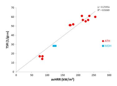
Figure 8. Total smoke release in  $m^2/m^2$  per gram of EVA versus average HRR for various EVA filled with ATH and MDH.
