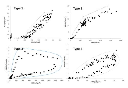
Figure 1. Various RSR versus HRR curves for different materials (type 1—PE; type 2—DGEBA-type epoxy; type 3—PA6; type 4—PE filled with 10 wt% of -TBBPA).
