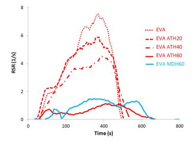
Figure 6. RSR versus time curves from cone calorimeter tests for pure EVA and EVA filled with mineral fillers.
