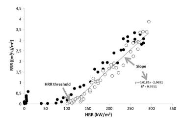
Figure 2. RSR versus HRR curve of PE with two parameters investigated in this work: slope A and HRR threshold (HRR $_{
