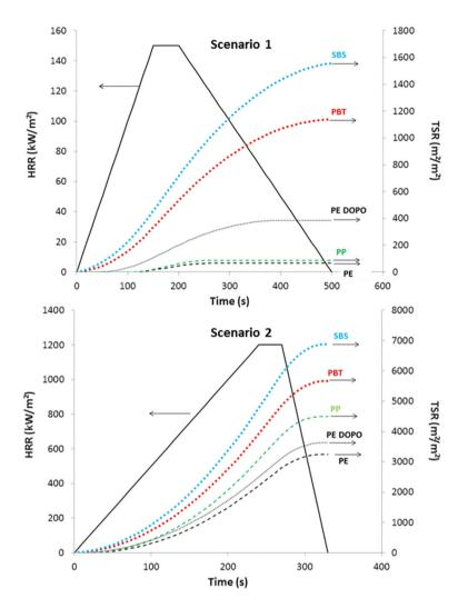
Figure 12. Total smoke release for different materials for a low burning rate scenario (scenario 1) and for a high burning rate scenario (scenario 2).
