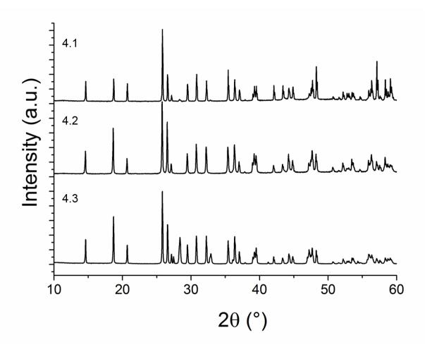
**Figure 3.** PXRD patterns collected for the samples prepared by the three varieties of "hydroxide precipitation" route (4). U(IV) + Ti-alkoxyde (4.1), with addition of 3 mol.% excess of titanium (4.2), with addition of Ti-alkoxyde after basification (4.3).
