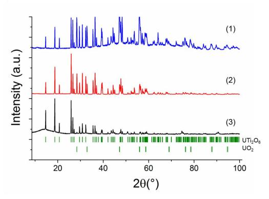
**Figure 2.** PXRD patterns obtained for brannerite samples prepared by "acetate route" (1), "alkoxide/nitrate route" (2) and dry chemistry route (3)
