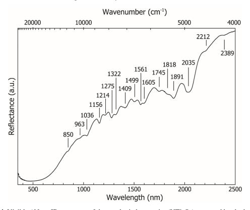
Figure 4. Visible / Near-IR spectrum of the synthetic brannerite ( $UTi_2O_6$ ) prepared by the hydroxide route (4.2). The position of the spectral features are expressed in nm.
