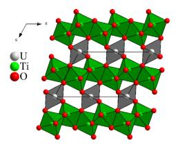
Figure 1. Representation of the crystal structure of UTi<sub>2</sub>O<sub>6</sub> down the b axis
