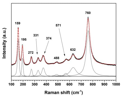
**Figure 5.** Raman spectrum of single-phase synthetic UTi<sub>2</sub>O<sub>6</sub> brannerite obtained by "hydroxide precipitation" (4.2), i.e. in the presence of 3 mol.% excess of titanium in the starting mixture.
