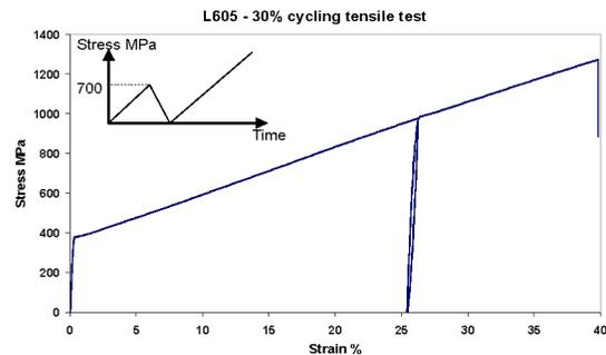
**FIGURE 5.** Stress-strain curve of the L605 cycling test.
