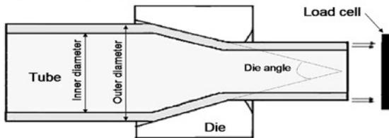
FIGURE 2. Hollow sinking
