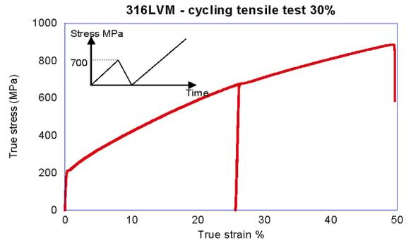
**FIGURE 4.** Stress-strain curve of the 316LVM cycling test.
