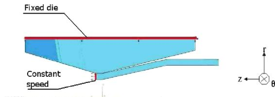
FIGURE 6. Boundary conditions of the drawing process model.
