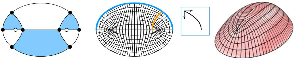
**Figure 11.** A result of an optimisation procedure: the shell structure is a Marionette Mesh (top view and prescribed curves on the middle) minimising total elastic energy. On the right: red areas indicate compression.
