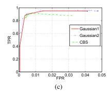
FIGURE 3. The segmentation of piecewise Gaussian distributed signal. (a) shows the hit rates with respect to the SNR. (b) shows the normalized  $\ell_2$  reconstruction error with respect to hyperparameter at a low SNR scenario (SNR = 10), and (c) shows the corresponding ROC at this scenario.
