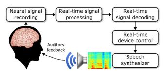
Fig. 1. Principle of a speech brain-computer interface.
