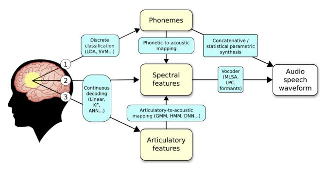
Fig. 4. Three representations of speech (phonetic, acoustic or articulatory) can be decoded from brain signals, each implying the use of specific speech synthesis techniques to build a speech BCI.
