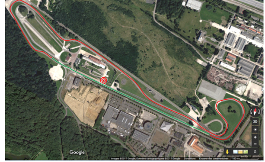
Fig. 6. Versailles-Satory test track (green line = RSU coverage)
