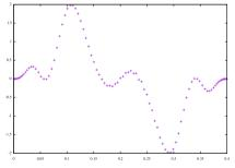
Fig. 7. Inflow perturbation  $(\sigma(\boldsymbol{\xi}_1, \mathbf{p}_{\boldsymbol{\xi}^1})\mathbf{n}.\mathbf{n} \text{ versus } x_2)$ .
