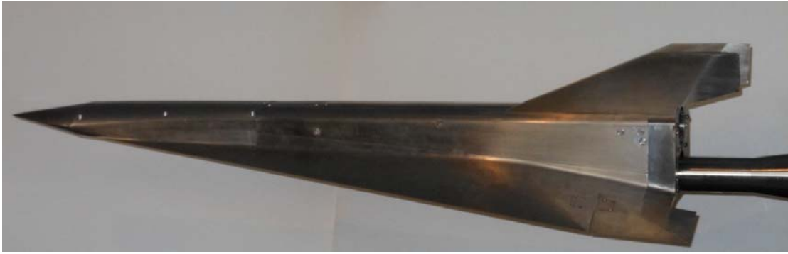
Fig. 18. The model of the ETV Glider Option mounted on a sting.
