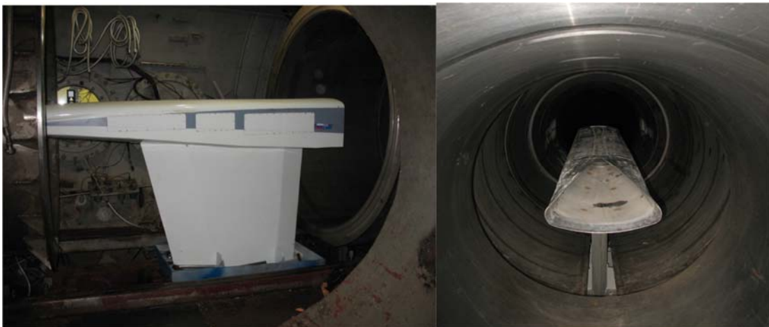
Fig. 42: Low thermal heat inertia scramjet module installation in the CIAM free-jet facility.
