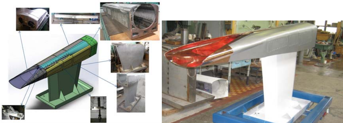
Fig. 41: The full-scale EFTV scramjet module with low (left) and high thermal heat inertia (right).
