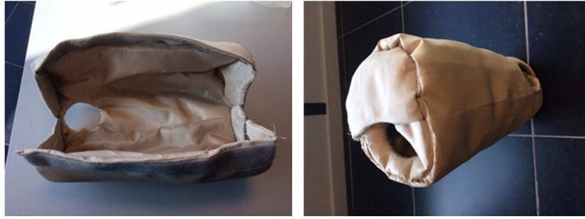
Fig 14. Aeroguard 160 ® based jacket of the actuators
