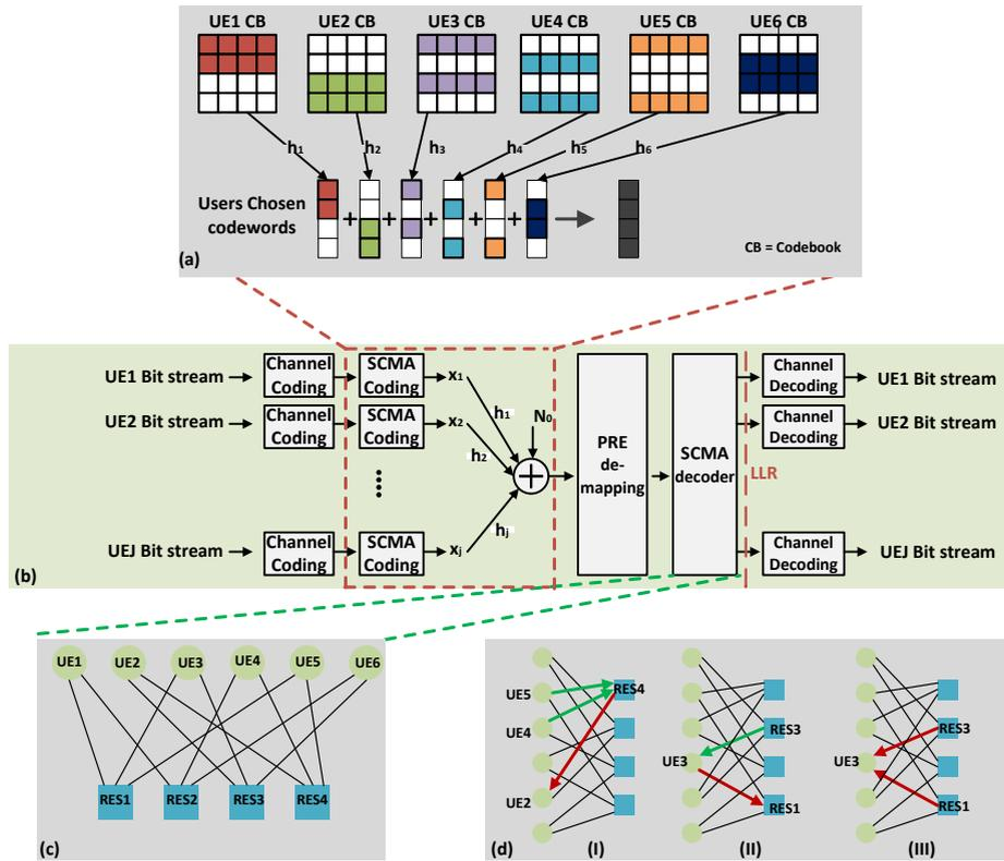
**FIGURE 1:** a) SCMA encoder with 6 users (layers) and 4 physical resources, b) SCMA uplink chain with channel coding, c) Factor graph representation of a decoder, d) Message Passing Algorithm based on Bayesian factor graph: (I) Resource to user message, (II) Guess swap at each user and user to resource message, (III) Final guess at each user.
