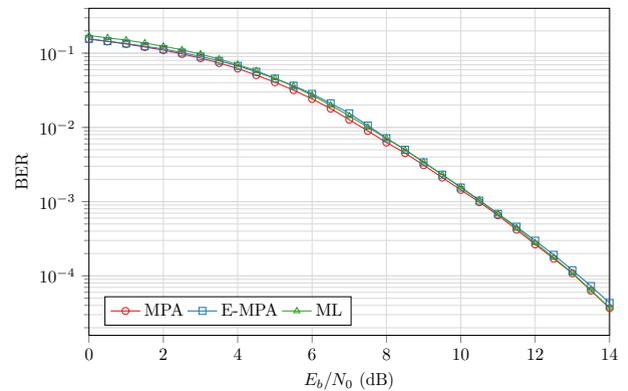
(a) BER performance comparison of ML, MPA and E-MPA for 5 iterations.
