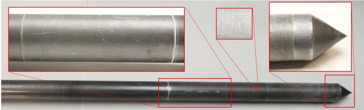
Fig. 5. Simplified cross-section and view of the instrumented pile-probe
