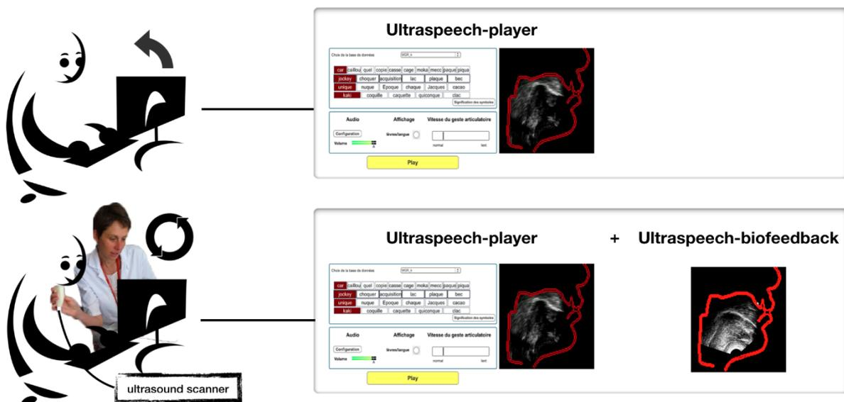
**Figure 1.** Top: illustration of the control interface and midsagittal ultrasound image display with sketchy vocal tract outline provided by *Ultraspeech-player* and used in the *IL* protocol. Bottom: illustration of the double interface, including the real time display of the speaker's tongue by *Ultraspeech-biofeedback*, used in the *FB+I* protocol.
