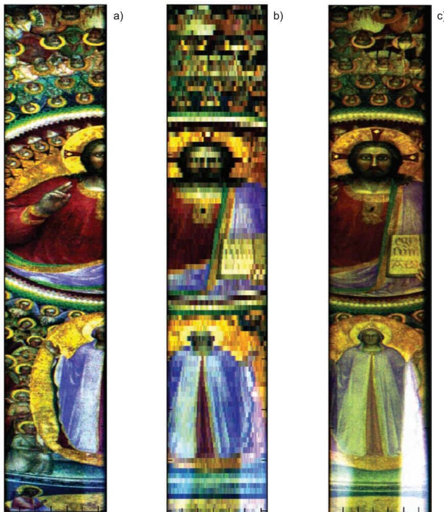
Figure 2 – a) RGB reconstruction from scan IMG2_R (reflectance image, 600 lines) with spectral channel at 600 nm, 500 nm, 400 nm ;b) RGB reconstruction of a very low resolution scan IMG3_R (reflectance image, 100 lines) with spectral channel at 600 nm, 500 nm, 400 nm; c) RGB reconstruction from scan IMG4_R (reflectance image, 600 lines) with spectral channel at 600 nm, 500 nm, 400 nm.
