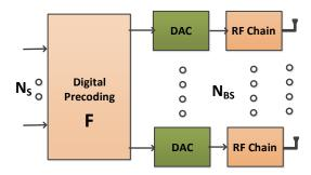
Figure 1: The fully digital beamforming architecture.
