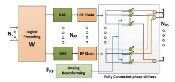
Figure 2: The fully connected HBF architecture.
