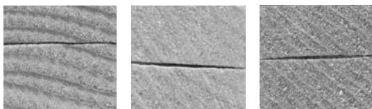
Figure 1 – Fungal pigments applied via pressure treating. Left: Abies procera with the green stain of Chlorociboria spp.; middle: Pinus contorta with yellow stain of Scytalidium ganodermorphothorum ; right: Pinus contorta with the pink stain of Scytalidium cuboideum
