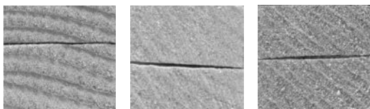
Figure 1 – Fungal pigments applied via pressure treating. Left: Abies procera with the green stain of Chlorociboria spp.; middle: Pinus contorta with yellow stain of Scytalidium ganodermorphothor ; right: Pinus contorta with the pink stain of Scytalidium cuboideum
