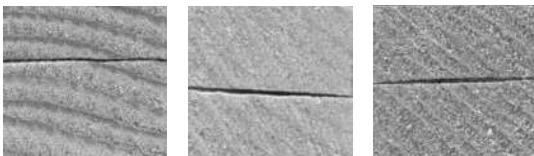
Figure 1 – Fungal pigments applied via pressure treating. Left: Abies procera with the green stain of Chlorociboria spp.; middle: Pinus contorta with yellow stain of Scytalidium ganodermorphothorum ; right: Pinus contorta with the pink stain of Scytalidium cuboideum
