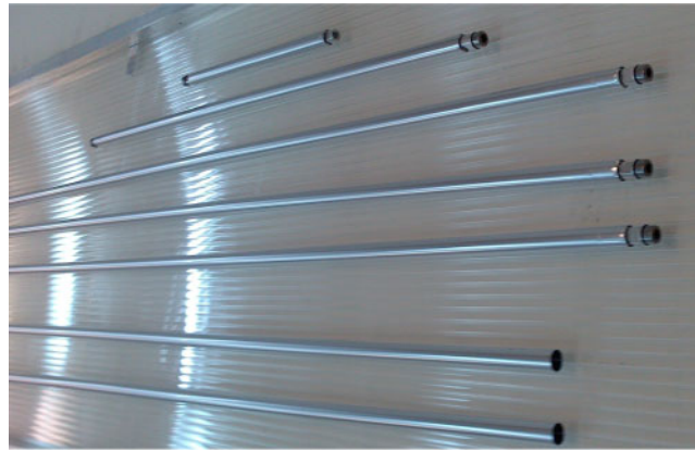
Fig. 50. Sample tubes with 20 \mu\text{m} -thick walls with 70 nm-thick aluminum layers.
