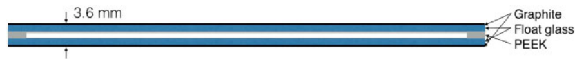
Fig. 76. Single-gap GRPC made of two layers of float glass, glued together using 1.2 mm PEEK spacers. On the outer part of the glass sheets, resistive paint (graphite-based) is used to apply an electric field of about 6.5 kV/mm across the gap. A mixture of a gas with high fluor content (forane) and a quencher ( \text{SF}_6 ) at a ratio of around 98:2 is flushed permanently through the chamber at a low rate of about 15 cc/min.
