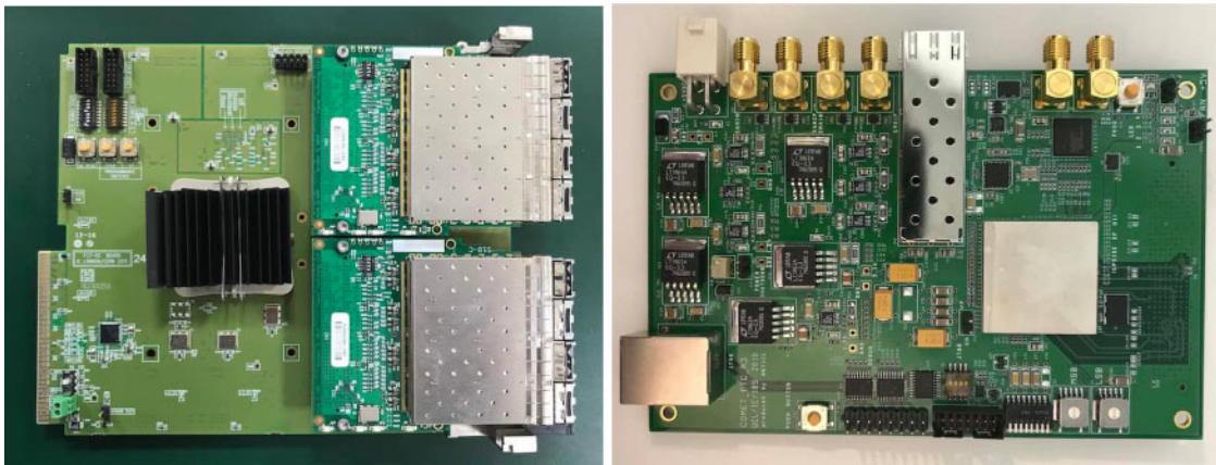
Fig. 79. (Left) FC7 board developed for the CMS experiment and adopted as the central trigger processor board in the COMET trigger system. An FPGA for trigger processing and board control is located at the center, and two commercial mezzanine cards for connecting subdetector trigger system are mounted on the right side of the board. (Right) Custom-designed FCT board for interfacing with the FC7 board.
