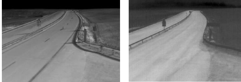
Fig. 11. Road marking observation in the LWIR spectral band during day sunny condition (left) and day rainy condition (right)
